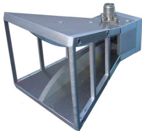
Fig. 2. Double ridged antenna (4-40 GHz).
