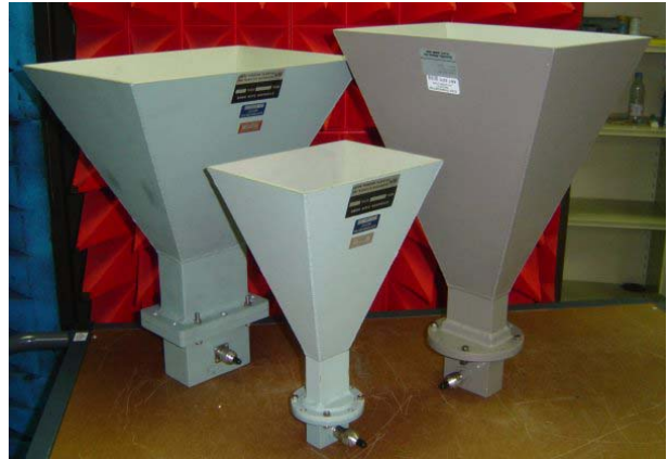
Fig. 5. Calibrated Standard Gain Horns from the DTU-ESA Spherical Near-Field Antenna Test Facility.
