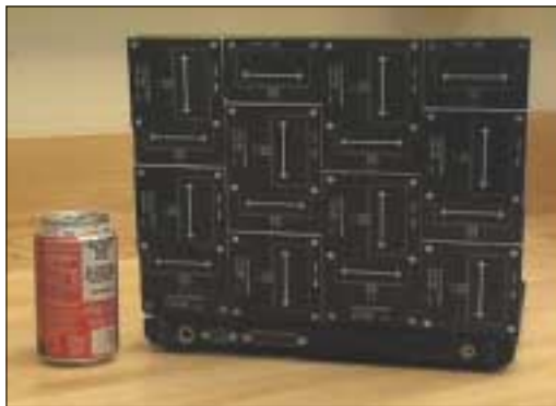
■ Figure 9. A terminal with 16 antennas mounted on a laptop.
